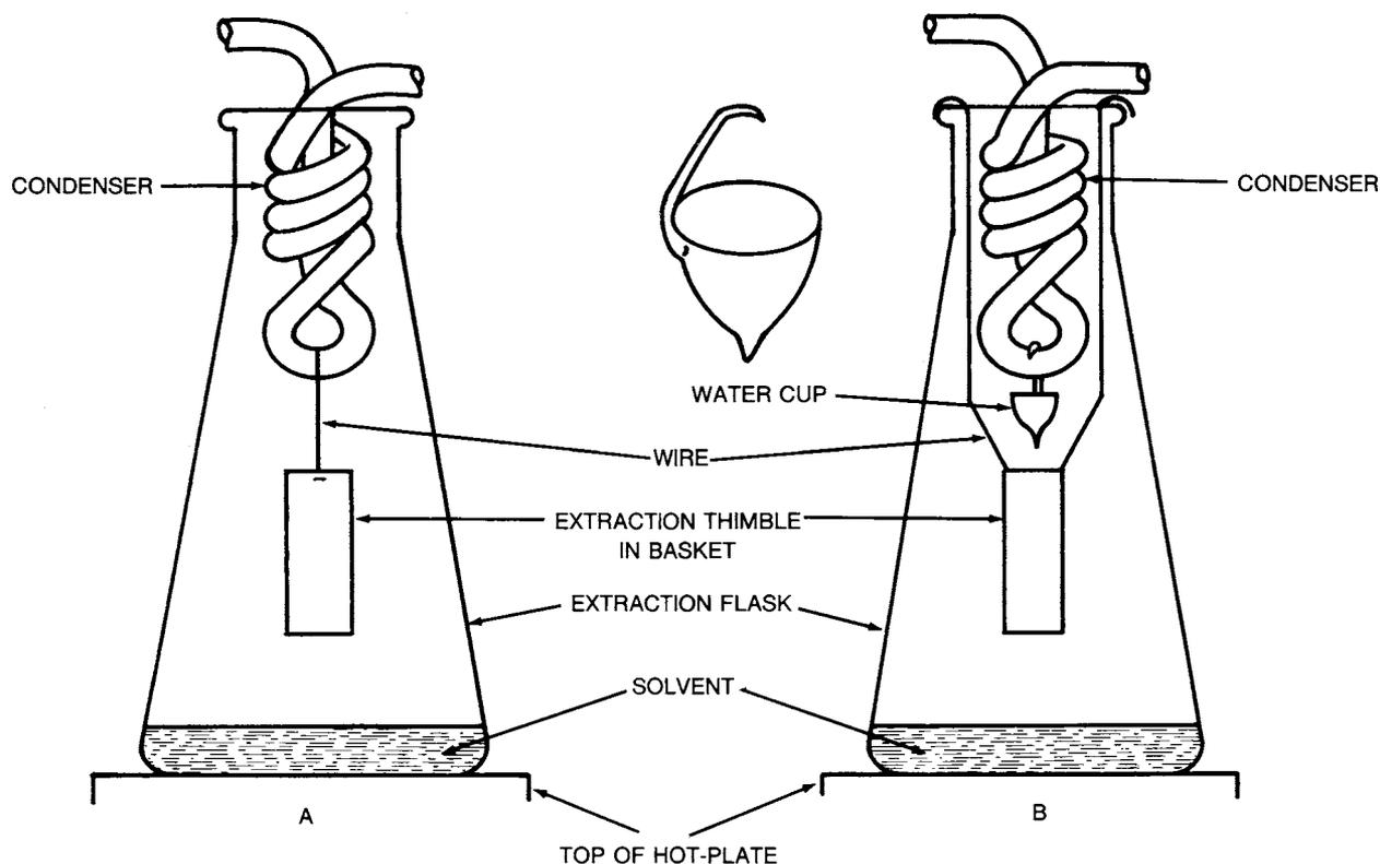
NOTE—Apparatus B shows the water cup in position.
