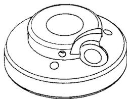
FIG. 9 Crucible Cover (Detail 2 of Fig. 7)
