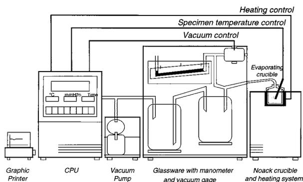
**FIG. 6 Automated Non-Woods Metal Noack Evaporative Apparatus**
