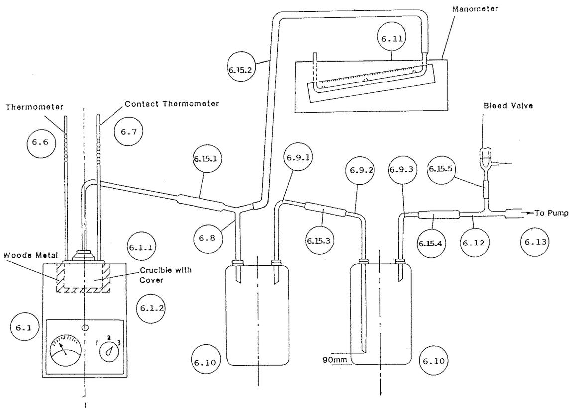
FIG. 5 Test Apparatus
